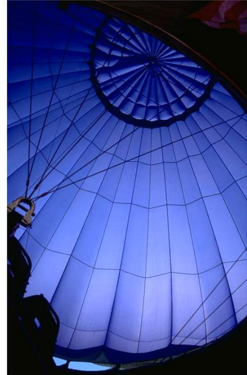
To make the balloon rise, the pilot turns the burner up. The flames heat the air. To make the balloon go lower, the pilot turns the burner down so the air cools.
